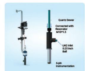
Liquid Nitrogen Variable Temperature System 93-573 K
