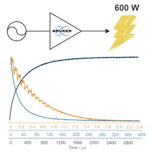
Different relaxation time measurements of a solid nitroxide sample with the 600 W SSA.
