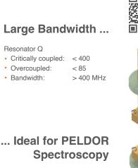
The large bandwidth and conversion factor ensures large modulation depths in PELDOR/DEER experiments.
