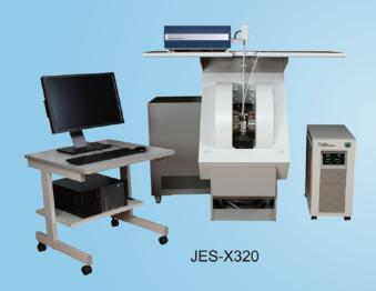
JEOL' s ultrahigh sensitivity ESR have evolved into full computer-controlled model equipped with a high stability microwave source and field control system.
