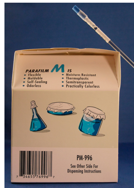
Sealing caps of sample tubes during cryogenic applications prevents the cap from popping off.
