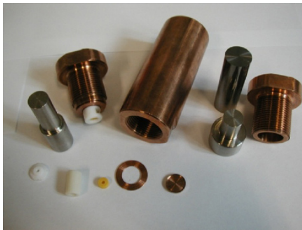
Fig. 6. Components of the high-pressure EPR cell enabling low-temperature measurements at pressures up to 18 kbar.
