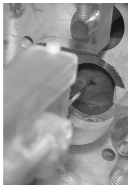
Fig. 1. Oxylite™ probe, mounted in the stereotactic frame, penetrating the FSa tumor in the hind leg of a C3H mouse immobilized in the EPR resonator. The Oxylite™ probe was advanced to the length of the tumor. Spatial coordinates of probe tip can be controlled within 1 millimeter accuracy. For scale, the diameter of the tumor bearing inductive element of the resonator (the hole through which the tumor bearing leg extends) is 16 mm. In an example of an x-ray of the Oxylite™ location in the tumor, it is seen curving away from the direction of the needle used to penetrate the animal skin [19].
