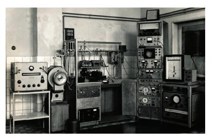
Figure 1. The first EPR spectrometer in Slovakia built in 1959.
