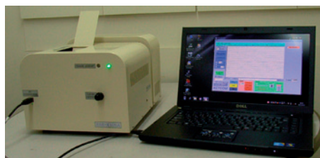
Potable ESR instrument : ESR-X10SB
