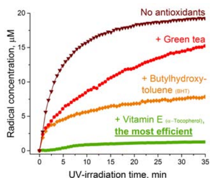
Figure 2. Evaluation of antioxidants' effect on a skin care product during UV-irradiation shows vitamin E to be the most efficient antioxidant. The data were collected with a Bruker EMXnano EPR spectrometer equipped with a light guide for in situ photochemical reactions. The concentration was determined with the SpinCount module.
